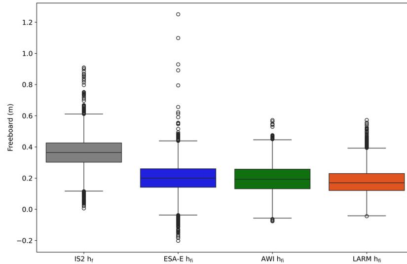
Fig. 2: Boxplots of total freeboard ( $h_f$ ) for IS2 and the ice-only freeboard ( $h_{fi}$ ) for the ESA-E, AWI, and LARM products.
