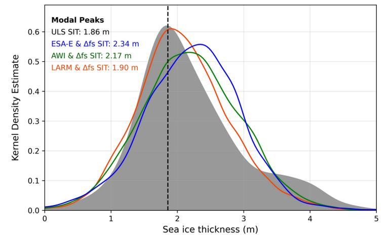
Fig. 5: Kernel density estimates of daily mean SIT for ULS and total Cryo2Ice SIT distributions using ESA-E, AWI, and LARM over 2020-2022. The shaded region is the ULS distribution used for validation, and the dashed line corresponds to its modal peak.
