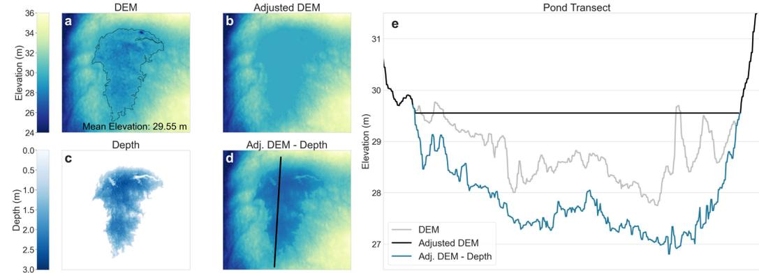
**Figure 2** – Steps used to calculate depth and bathymetry for Pond 1: (a) DEM with pond marginal pixels and mean marginal elevation in black, (b) adjusted DEM with smoothed water surface equal to the mean marginal elevation, (c) water depth calculated from WV-2 reflectance (Table 2), (d) pond basin bathymetry, calculated by subtracting water depth from the adjusted DEM, with ICESat-2 transect in black, and (e) profiles of pond data in a, b, and d along an ICESat-2 transect.
