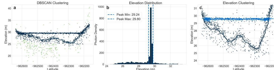
**Figure 3** – Steps used to calculate depth and bathymetry from ICESat-2 photons for Pond 1: (a) DBSCAN clustering to remove low density photons, (b) histogram of remaining high density photon elevations, and (c) clustering based on elevation histogram peak, with moving averages calculated for the air-water interface and the water-ice interface.
