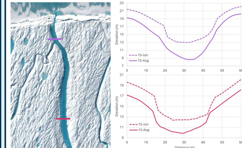
**Figure 7** – Channel bathymetry at two cross-sections of the Petermann river at the beginning (June 15) and end (August 15) of the 2016 melt season. Bathymetry is calculated from paired WorldView-3 imagery and ArcticDEM strips using the DC (B-G) method. Imagery © 2016 Maxar.
