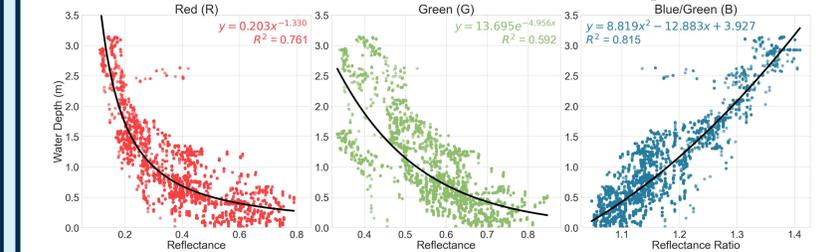
**Figure 6** – ICESat-2 derived depths vs. WorldView-2 reflectance in the red and green bands, and the blue/green band ratio, with best fit lines in black.
