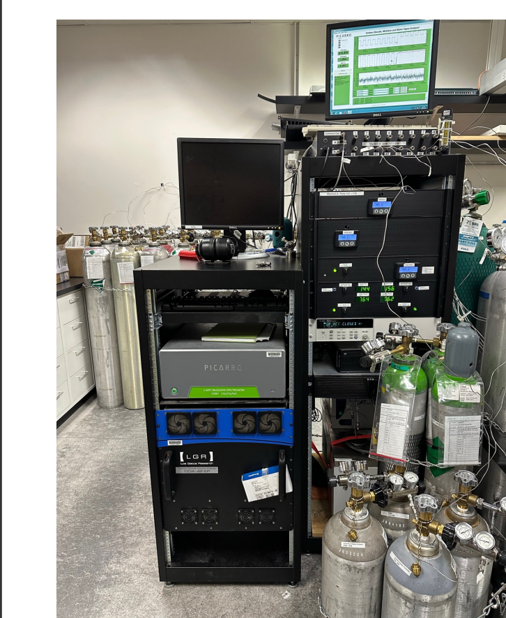
CO 2 and CH 4 Scale Transfer System
