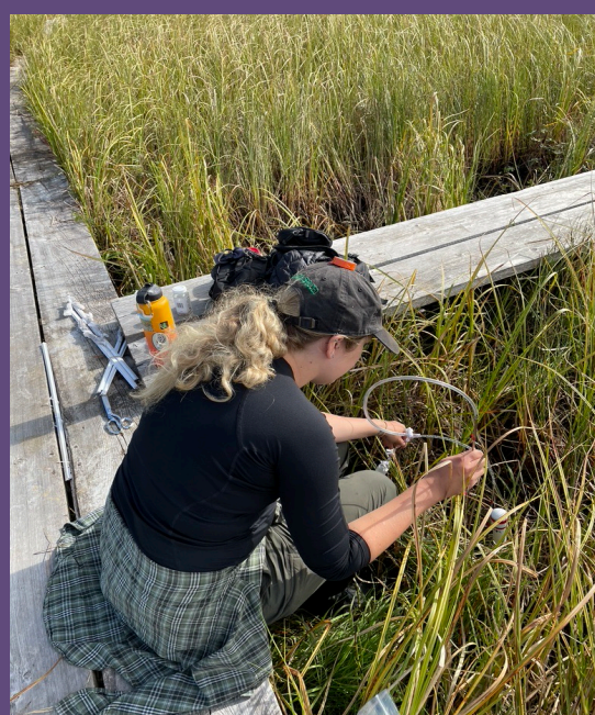
Fig. 3. Collecting porewater at the rich fen experiencing water-table manipulation during a dry summer.
