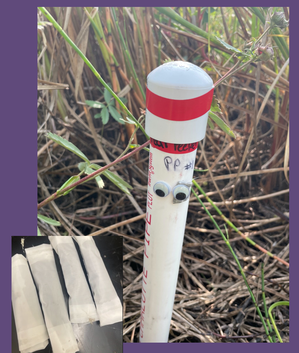
Fig. 9. Peat peepers are PVC pipe with holes drilled along its length to allow for exchange between the peeper and the environment. We place mesh packets of a common peat substrate at 10 cm depth increments to measure the effects of environmental, experimental manipulation on RAOM.
