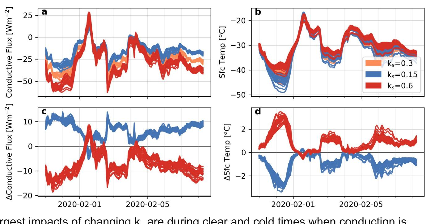
Largest impacts of changing k<sub>s</sub> are during clear and cold times when conduction is largest; smaller differences occur during warm cloudy periods.
