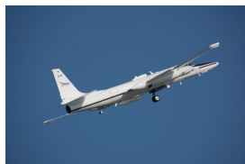
The NASA ER-2 on takeoff with the DCOTSS payload. UCATS is located in the upper Q-Bay, directly behind the cockpit. The sampling inlet for UCATS is visible on the bottom, forward of the landing gear. AWAS is mounted the "belly pod" aft of the wheel, with other instruments located in the nose, wing pods, and Q-Bay.
