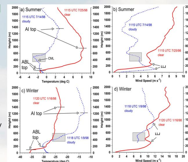
**Figure 1:** Sample temperature and wind profiles in the lowest 2 km at the SHEBA site for a), b) summer and c), d) winter for clear (solid) and cloudy (dotted) conditions. The shaded grey region represents the observed clouds for the respective soundings. The Arctic inversion tops (AI), the atmospheric boundary layer tops (ABL), the cloud mixed layer (CML), and the low-level jets (LLJ) are given for each profile. (from Persson and Vihma 2017)
