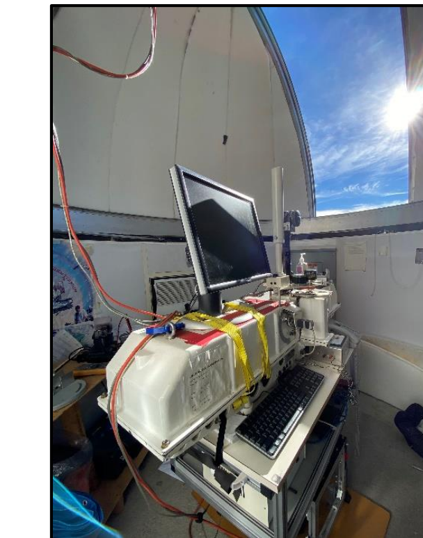
Dobson Spectrophotometer at NOAA ESRL - Boulder, CO (credit: Peter Effertz)
