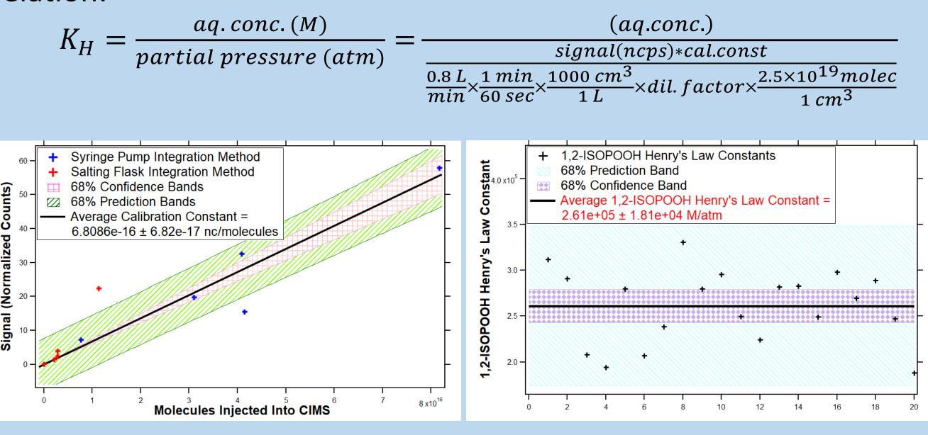
Integrated signal vs number of molecules injected.
