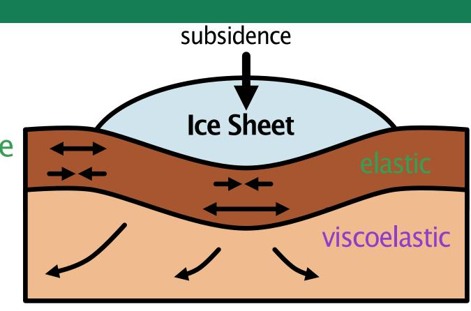
Schematic of the different forms of solid Earth deformation caused by ice sheet loading
