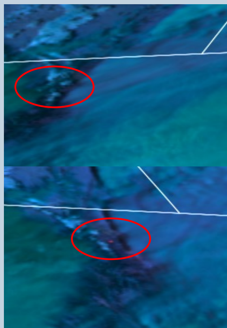
Figure 1: Fire product from GOES East (top) and GOES west (bottom) from Kruger Rock Fire Nov 16 2021 show cloud and/or smoke blocking have impacts on FRP detection. Images both taken at 19:30 UTC. GOES East does not show a sign of FRP and GOES west does.
