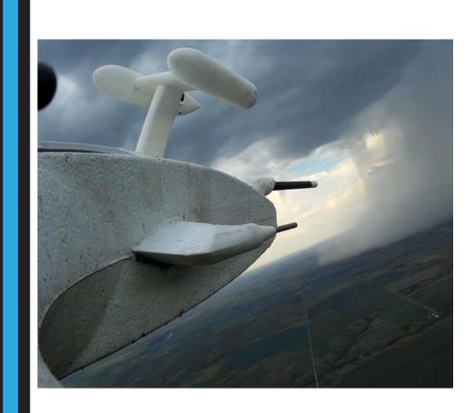
Pushing Boundaries: Environmental science related deployment of UAS requires that aircraft are hardened to withstand a variety of conditions. This includes operation in extreme temperatures, various modes of clouds and precipitation, at extreme altitudes (both low and high) and through in corrosive environments. IRISS has worked with scientists to advance systems to ensure reliable performance of aircraft and sensors in a range of operating environments.
