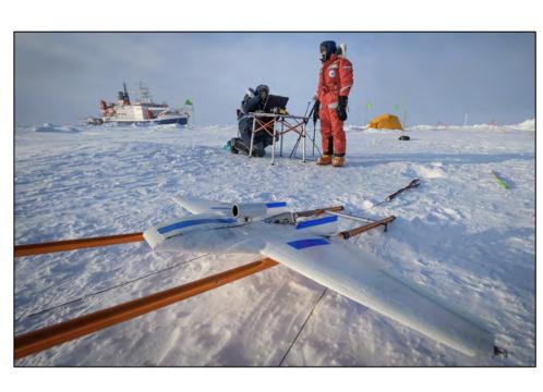
Autonomous and Coordinated Flight **Capabilities:** IRISS is working to advance aircraft control and coordination systems to support different sampling modes, including high-altitude sampling as done with the NOAA GML HORUS platform. This includes enhancing onboard decision making to allow aircraft to autonomously optimize sampling of features of interest, and to support "swarming", or coordinated flight of a fleet of aircraft.
