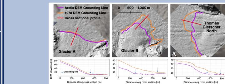
Figure 3. Grounding lines of the HFIS tributary glaciers determined by the distinct break in slope. The DEMs have been adjusted for the EGM2008 geoid and the 3.85 m bias. The background is the 1978 DEM hillshade extracted in 2.5 km boxes (Fig. 4).
