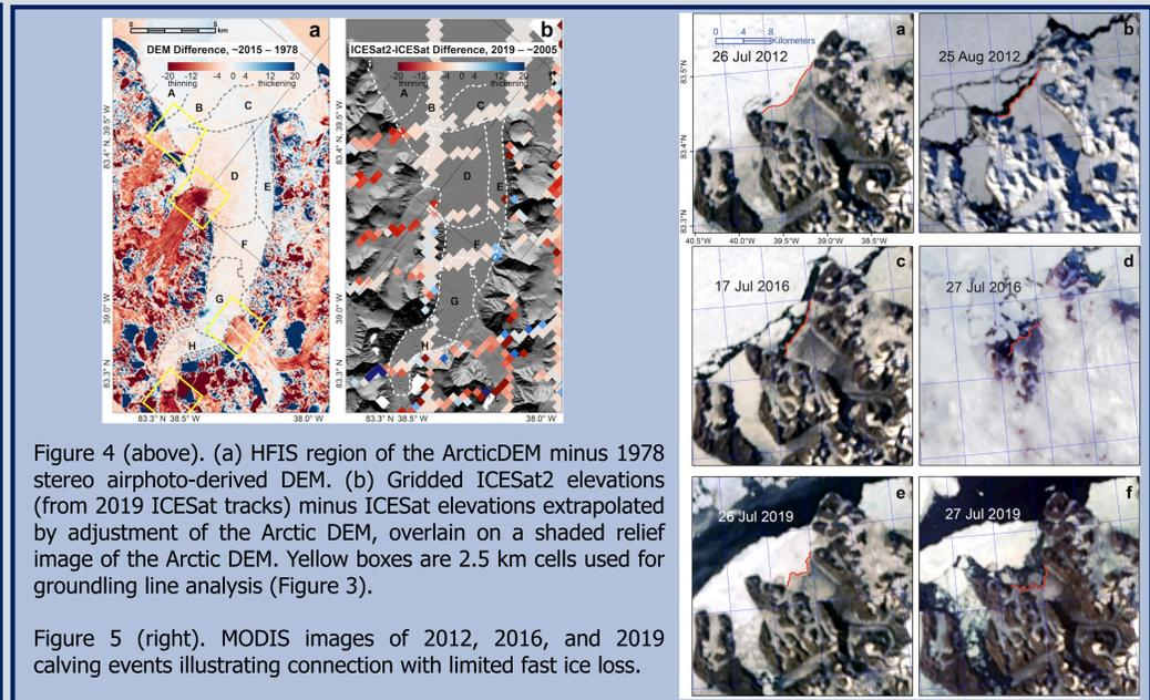
Figure 4 (above). (a) HFIS region of the ArcticDEM minus 1978 stereo airphoto-derived DEM. (b) Gridded ICESat2 elevations (from 2019 ICESat tracks) minus ICESat elevations extrapolated by adjustment of the Arctic DEM, overlain on a shaded relief image of the Arctic DEM. Yellow boxes are 2.5 km cells used for grounding line analysis (Figure 3).
