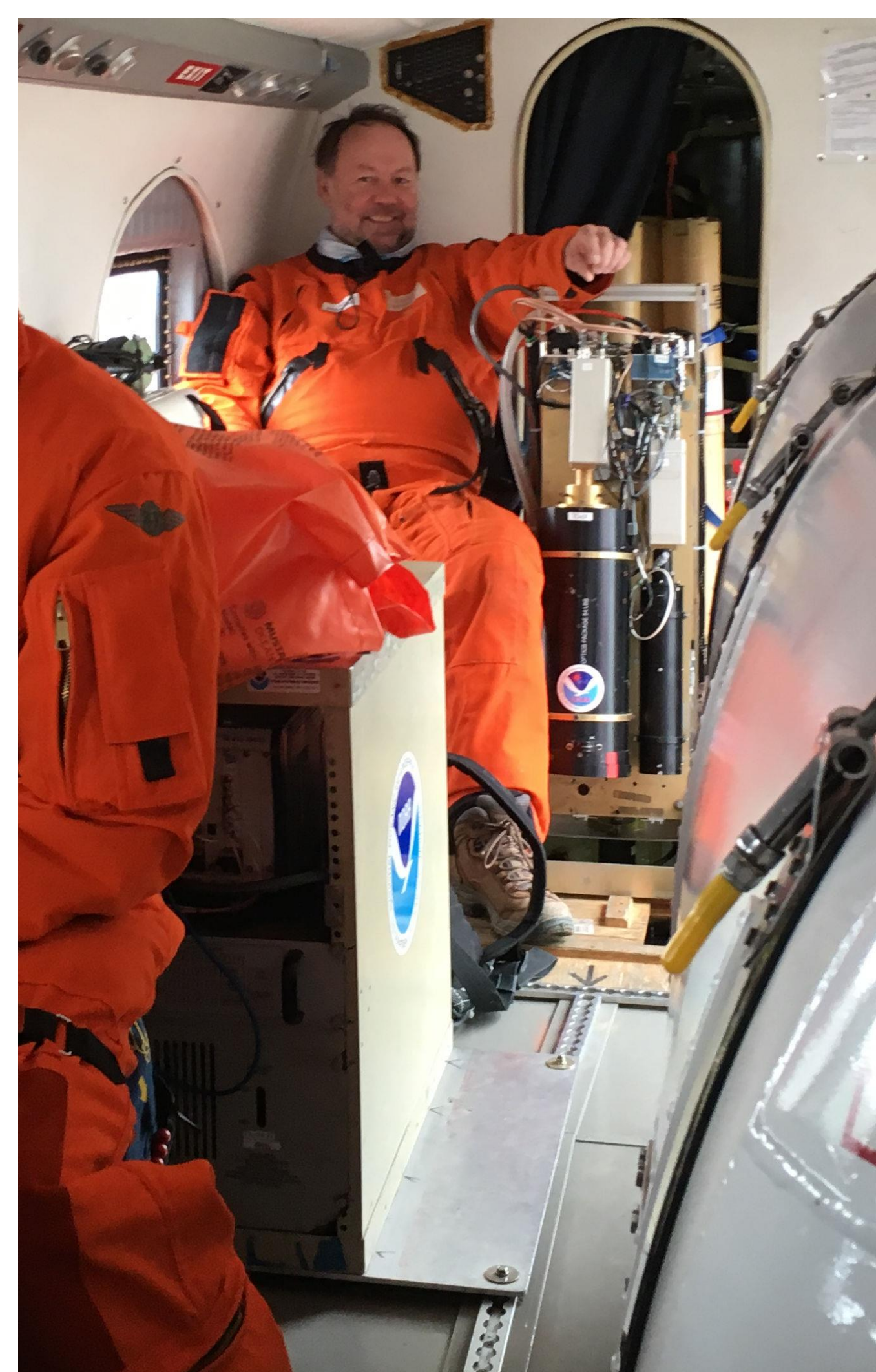
Photo of lidar optics package in rear of NOAA Twin Otter and electronics rack in front of operator (Marchbanks). Both lidar components can be identified by NOAA stickers.
