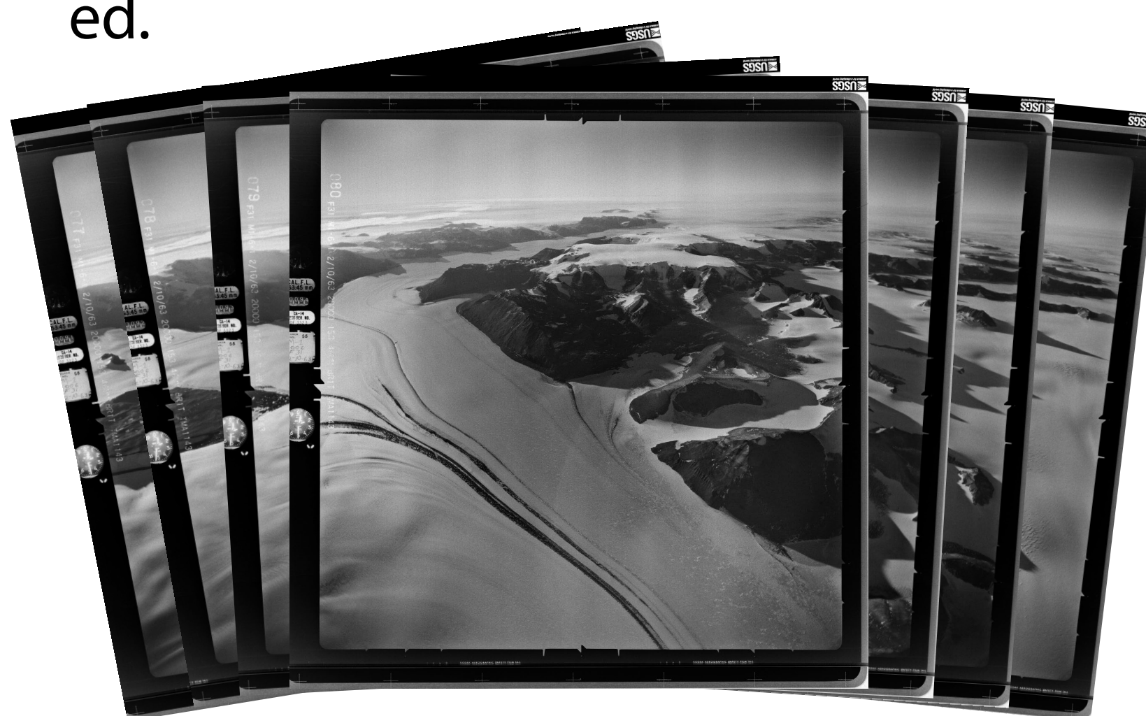
Figure 2: A set of oblique TMA images overlooking Shackleton Glacier, collected in 1960. We use both oblique and vertical images in the SfM photogrammetry processing. Results from entire extent (7 x 7 km) of the vertical (0° nadir) photos were used, but only rendered a distance of ~20 km of the oblique image results.
