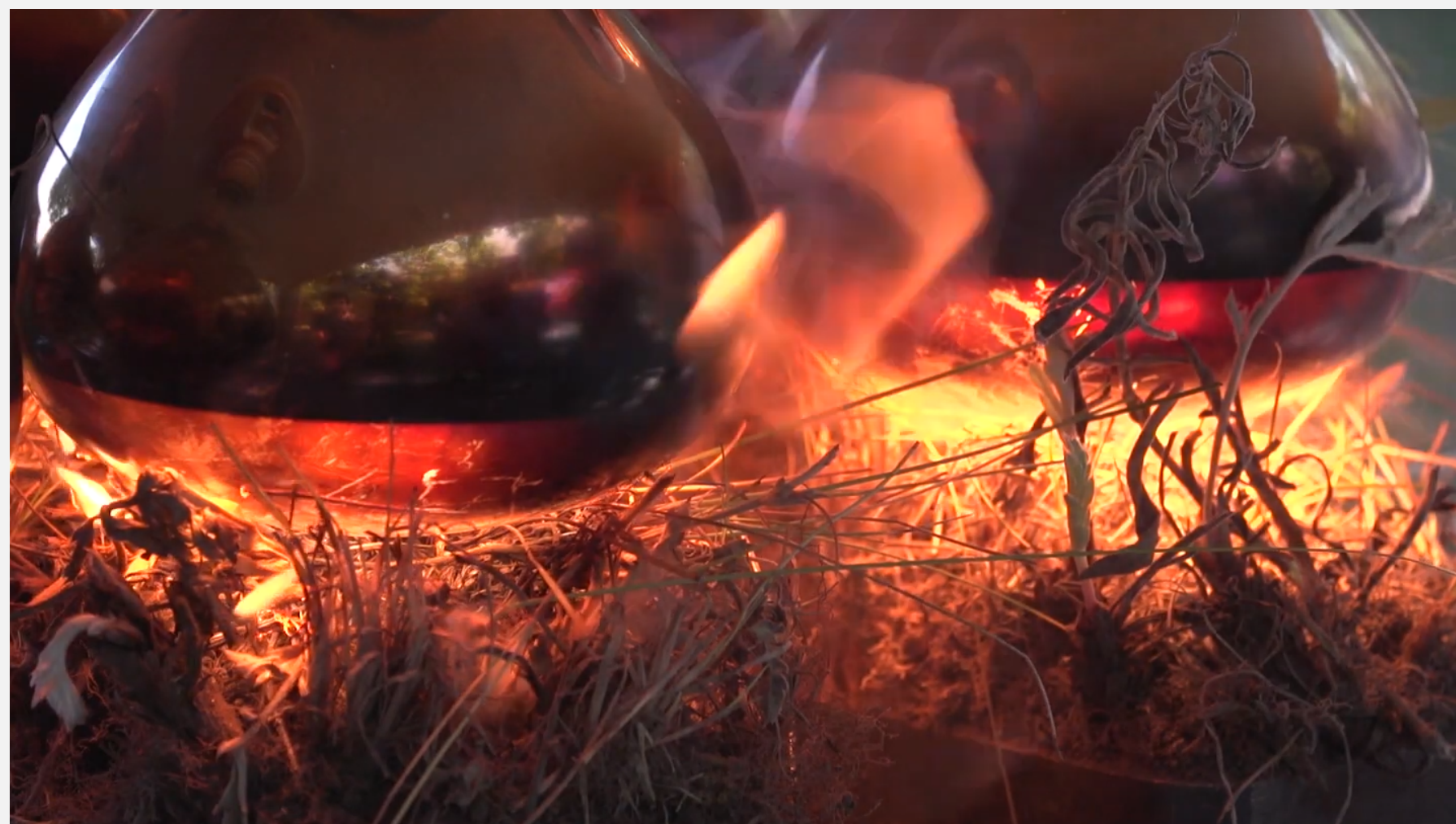
Figure 3: Wildfire simulator using heat lamps to burn the surface of the soil samples
