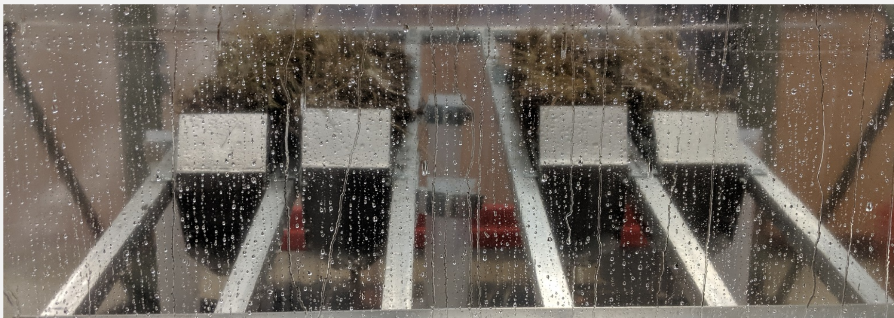
Figure 4 (above): Tilting mechanism and funnel setup in the rainfall simulator
