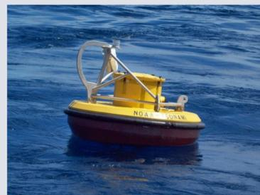
The DART system, operated by the NOAA National Data Buoy Center (NDBC) and other international partners, is a global array of 62 offshore bottom pressure recorders (BPRs) which detect the tsunami by increased pressure from the wave passing over. Data are transmitted to a nearby surface buoy, which relays the message to tsunami warning centers via satellite that a tsunami is on the way.
