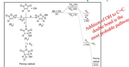
Values in parentheses are barrier heights (in kJ mol<sup>-1</sup>) calculated using CBS-QB3 method
